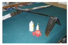
Make sure you have **grinded the gluing spots** on fuselage and V-tail thoroughly, before you glue.
