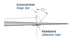
Now, place the V-tail on the boom. Before you glue it, Check the **alignment of the V-tail** regarding the axis of the fuselage and the **EWD**, so that it is fixed correctly.
