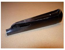
Push the boom into the middle part of the fuselage, until the boom stands out 400mm. If the boom can't be pushed out far enough, you can sand off some material inside the middle part of the fuselage.
