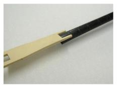
Before you glue the boom, check that the **servoboard** can be **fixed to the boom** inside the fuselage later according to the picture. The flat side of the boom should be on the upper side, the round one on the downside.
