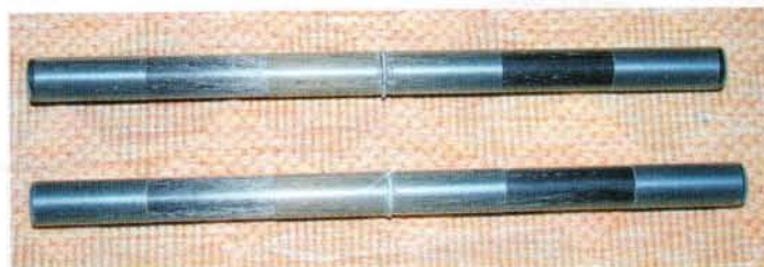
ABOVE LEFT: Carbon is difficult to photograph - here shown are my home-brew rear servo mounts for the HS 82 MGs. ABOVE CENTRE: HS 82 MGs fit perfectly and provide one answer to the tail end actuator choice. ABOVE RIGHT: All neatly installed - HS 5125 and its associated wiring - shown here is the flap servo. BELOW LEFT: Two very strong carbon joiners hold the wing halves together. BELOW RIGHT: Nose ballast was cast in two halves and then dressed to fit the nose.
