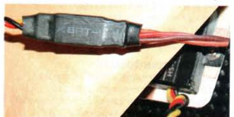
ABOVE LEFT: Epoxy-glass horns are employed throughout. ABOVE RIGHT: HS 5125 digital wing servo in place - do heat-shrink your extension leads - you know it makes sense! BELOW LEFT: The best solution by far for wing-mounted servos - Cubitts mounts (see text)! BELOW RIGHT: Lovely little HS 82 MG servo - perfect for the tail end. BOTTOM: The main wing root with joiner tubes - it's all carbon!
