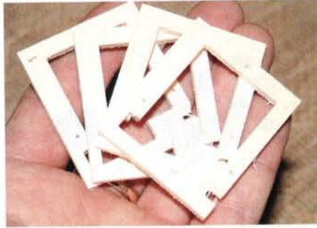
ABOVE LEFT: HS 5125 and JR DS 161 servos are virtually identical (same gearbox and case) so either will fit! ABOVE RIGHT: Supplied ply servo mounts were perfect for HS 125, 5125 or DS 161 wing servos.
