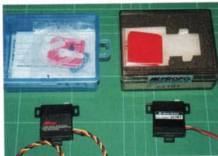
ABOVE LEFT: HS 5125 and JR DS 161 servos are virtually identical (same gearbox and case) so either will fit! ABOVE RIGHT: Supplied ply servo mounts were perfect for HS 125, 5125 or DS 161 wing servos.
