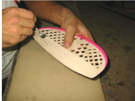
(Glue for indoor foil is applied.)
