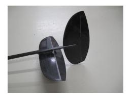
Vertical stab for right handers: has the hinge line on the left (seen in flight direction), see 3<sup>rd</sup> picture **Vertical stab for left handers:** has the hinge line on the right (seen in flight direction), see 3<sup>rd</sup> picture
