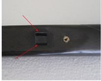
During flight you should control that the **screws are always firmly screwed**. It could happen that the contacts slip to the black plastic strips and the spring contacts raise from the contact areas. So please **level the plastic strips to the contact areas**. So lifting off from this areas should be avoided.
