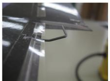
Open the hole of the lever to have a good fitting without much friction and without getting too much clearance.
