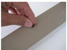
**Isolate all the contacts** that should not touch the carbon. A contact to the carbon could cause failures to the controls.
