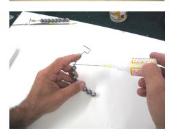
Insert the ballast through the left opening of the fuselage **into the ballast tube**.
