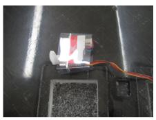
When you want to **replace the servo**, you just have to **cut the shrinking tube** and take out the servo.
