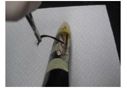
Place carbon rovings at the left and right and the upper and lower side of the radio board.
