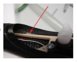
You can fill the **glue into a small plastic bag** and cut a whole on one corner. By this, it will be **easier to apply** the glue exactly.
