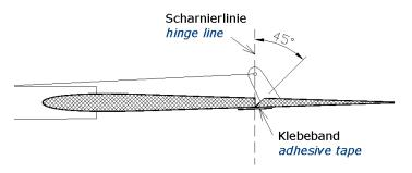
**Cut a slot** in the rudder in extension of the axis of the fuselage. It is advisable to leave the lower laminate uncut. Next, glue the **lever** into the slot. The **hole of the lever** should be located just **above the hinge line**.
