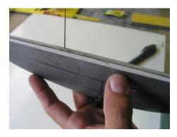
**Push the vertical stab** (first for a test) into the oval end of the boom **until ist stops**. Then check, if the stabilizer is **aligned correctly** to the wing.
