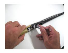
The **hook** of the ballast package is **locked in the servo board**.
