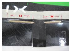
For easy and accurate applying of the glue use the **edge of a plastic bag**.
