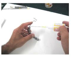
Insert the ballast through the left opening of the fuselage **into the ballast tube**.
