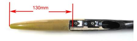
If necessary, the edges of the servo arms can be ground down a bit.
