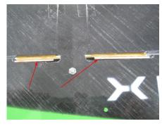
During curing of the glue put a **strip of tape** over everything to secure the correct position of the parts.
