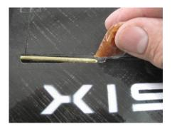
For holding the right position during the curing of the glue, prepare distance sheets. Use them under the tube and in front of the tube to place the tube as high as possible to the upper edge of the aileron. Note that there is enough space near the hinge to guarantee the free movement of the brass tube.
