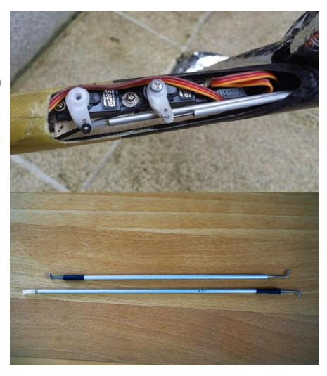
For this we need a special small ball connector and a handmade direct linkage made of aluminum tubes.
