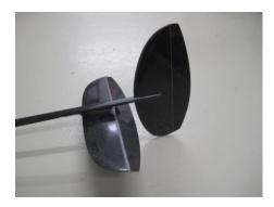
**Vertical stab for right handers:** has the hinge line on the left (seen in flight direction), see  $3^{rd}$  picture **Vertical stab for left handers:** has the hinge line on the right (seen in flight direction), see  $3^{rd}$  picture
