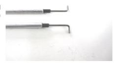
Push the steel hooks into the carbon tubes and the carbon tubes into the aluminium tubes. Grind all gluing spots and use epoxy glue for this bonding.
