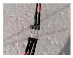
This is how the switch is made. Use a steel with 15mm length and a diameter of 0,5mm and bend it to U shape. Put a shrinking tube on it for better gripping. We recommend making more than one because these little switches like to escape ;-). During flight you can save the U-steel with tape.
