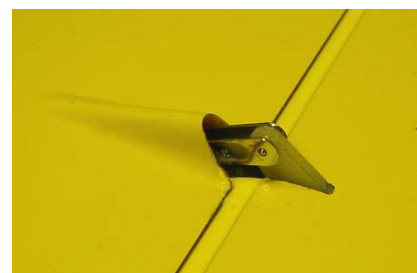
Connector for push rods, M2,5mm
