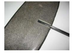
Last, glue the **two carbon covers** left and right of the join also with super glue. Note, that the hole for the installation of the elevator must be kept open.
