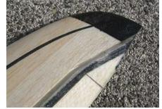
As you nearly don't recognize a damage of the leading edge of the wing (f.e. after hard landing), we advise to put a **strip** of adhesive tape over the leading edge.
