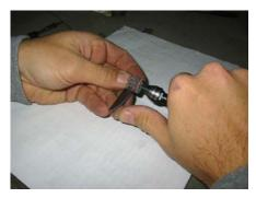
Lay the paper template on the wingtip and thrill a hole at the marked spot.
