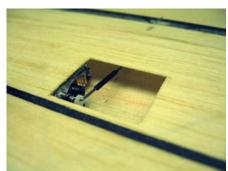
Hold the aileron in zero-position with a ruler. Now put a drop of super glue in the carbon pipe to fix the length of the pushrod.
