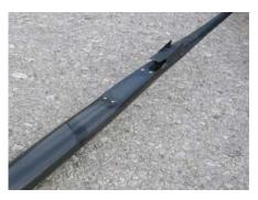
Firewor-X-tend fuselage with ready glued carbon tile.
