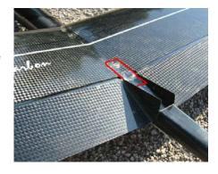
...or with the **little carbon tile** enclosed. Glue it on the part of the fuselage that is placed between the two ailerons.
