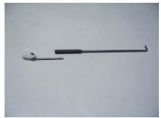
Drill a hole to lead the push rod through the wing and glue a plastic tube for better leading of the push rod.
