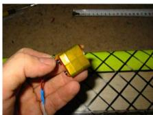
Glue the servo with Stabilit Express or with a 5minute Epoxy. Use a steel wire, d=1mm, as pushrod. You can make a variable joint by cutting the steel and gluing a piece of carbon pipe on one end.
