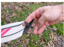
You should additionally strengthen the joint by forming a rim of glue. Use f.e. UHU 300 endfest oder Pattex Stabilit.
