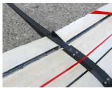
In order to move the triangular ends of the ailerons, you can bend a piece of **steel wire (1mm)** and glue it into the end of the aileron as shown. Let the wire jut out about 6mm. You can bend the end of the wire to ensure not to cause damage to the shell on the inside.
