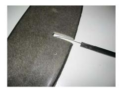
Then, **check** the **good fit** of the rudder. The axis of the boom should be right-angled to the hinge line of the rudder. The kevlar wire should not chafe on the sharp carbon. It must be free movable.
