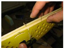
**Stick** the spring **into the balsa material** and then harden the balsa with super glue.
