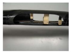
You can fix the servoboard with a drop of super glue to make the position check easier.
