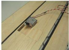
Shorten the lever of the servo, so that it can be moved inside the wing.
