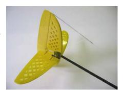
Another possibility is to lay the antenna **inside the gap of the aileron**. For improving reception on **carbon wings** you can solder the antenna to a steel wire, d=0,3mm, which you fix at the end of the wing and let stand out to the back about 10-15cm.
