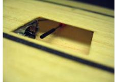
The **hole** in the lever should be a little bit in front of the turning axis of the rudder.
